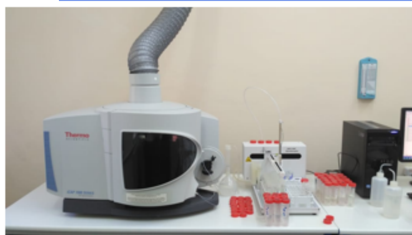
Determination of macro-elements in a sample using an ICAP 7400 Duo inductively coupled plasma emission spectrometer
