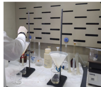
The process of radiochemical sample preparation
